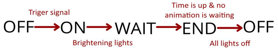
By default, each animation waits for an TRIG activation signal. When a signal appears on the input corresponding to a given animation (TRIG: I1, I2, I3, or I4), the animation switches to ON mode.
