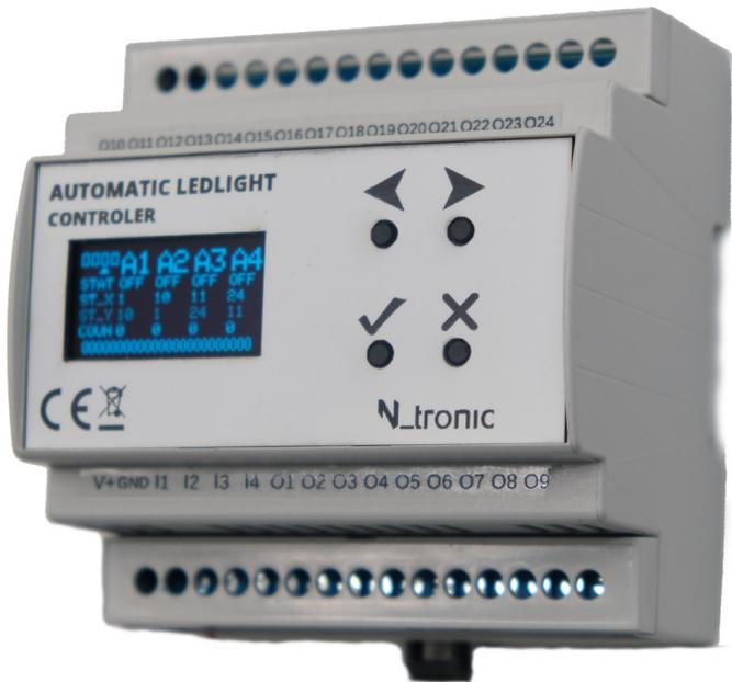
*AutoSteps24: 24 channel staircase lighting controller with four motion sensor inputs*
